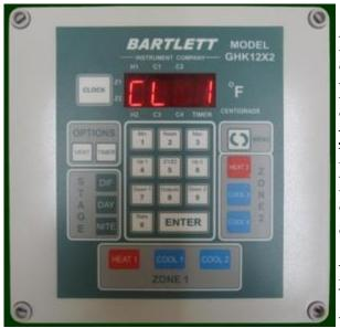
It's important to get your outputs programmed correctly so your greenhouse runs at an optimal level. If your outputs are not programmed properly, it could cause problems and the greenhouse may not heat or cool the way you want it to. The first step is to check your hysteresis setting, set all of your Cool outputs programmed (Cool 1, Cool 2, Cool 3, and Cool 4), and finally program your Heat outputs (Heat 1 and Heat 2).
