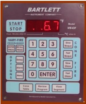
Here's a handy feature of Bartlett controllers that you may not be using! Did you know that you can use the 8 key on your V6CF and RTC1000 controllers to check which section of the kiln the controller is trying to heat. This can be a great diagnostic tool to help check whether the controller is functioning properly or if a relay or element has gone bad.
