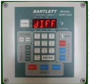
The 3 different growing stages on the GHK12X2 and RWL11X2 can be used to control your plant's height throughout the growing process. First, it's important to know the 3 stages - DIF, DAY, & NITE - and what they are used for.
