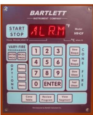
Did you know you can adjust the alarm settings on your controller before or during a firing to alert you at various temperatures? If you need to know when the kiln reaches its top temperature or different temperatures throughout the firing you can adjust it accordingly. When the alarm temperature is reached, a buzzer will sound but will have no effect on the firing itself.
