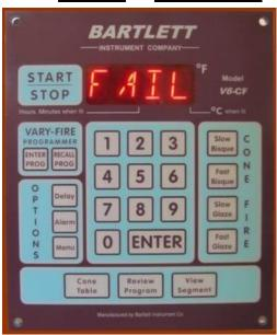
It is good practice to keep a spare thermocouple on hand when doing regular firings with your kiln. Stopping a firing or being unable to get your projects done because your thermocouple has malfunctioned can be very frustrating.
