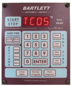
Thermocouple offsets are often used in zone controlled kilns to balance the heat work by either raising or lowering the temperature indicated by the thermocouples. This can be especially helpful if one zone tends to lag behind the other zones just a bit. It can also be used when a thermocouple is worn but is not yet ready to be replaced.
