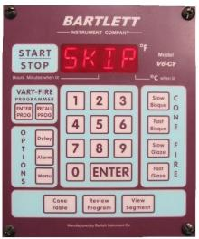
Skipping the remainder of a segment can be a helpful feature when firing your kiln, especially if it is the first time you are firing to a specific cone. If you check in your peep hole and see the cone has bent to maturity but your hold is not yet complete, you can skip to the next segment to begin a cool down segment sooner than originally programmed. This can prevent users from firing ware too long or at too hot of a temperature.
