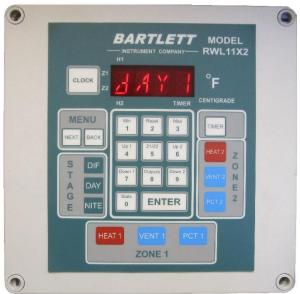
Bartlett controllers are designed to be a growing tool as well as a tool to precisely control temperature. That is why they also collect and store the temperature averages for the last 7 days. They store averages for DIF, DAY, NITE, and for the 24 hour period from the start of DIF to the end of NITE.
