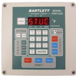
Getting a STUC error will cause the buttons on your controller to stop working until it has been remedied, so it's important to know what causes it and how to fix it. A STUC error indicates that one of the buttons is being held down for a prolonged period of time or is "stuck".
