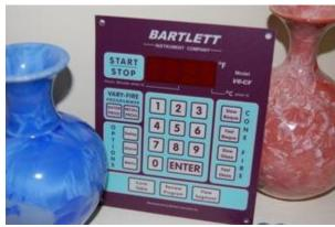
When an error code occurs, at times it can be worrisome but they are often helpful. An ErrP is an error that is meant to inform you of a brief or intermittent power failure. The controllers will only show ErrP when a firing is in progress, the kiln's temperature is higher than 140 degrees, and the temperature was changed by less than 250 degrees during the power failure. If there is a drop in temperature greater than 250 degrees, PF will be displayed and the firing will stop.
