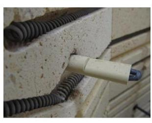
It is important to be mindful of your thermocouple placement during a firing. A properly placed thermocouple can make a big difference in accurate temperature readings. Follow these few tips for proper thermocouple placement in your kiln:
