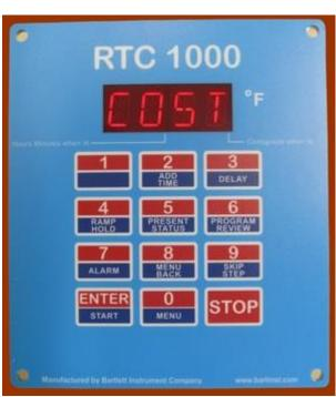
The RTC1000 has many great features, but did you know you could calculate the cost of firings? You just need to input two pieces of information (cost of electricity per kilowatthour and wattage rating of the kiln) into the controller and it will calculate it for you. The calculation will only be accurate if the correct information is added into the controller.
