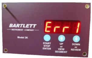
The Bartlett 3K controller displaying the "Err1" indicating the temperature isn't rising fast enough.
