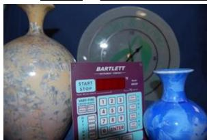
The diagnostics option on your Bartlett controller can be used to check each of the outputs on the kiln. By running diagnostics (dIAG), the controller will individually turn on each of the three outputs for one minute and 20 seconds starting with the top output. If there is an issue with your kiln, this is a good way of determining which output could be causing the issue.
