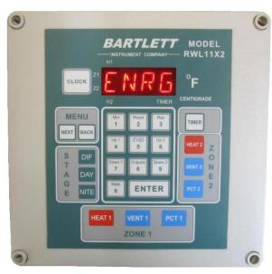
When using your proportional outputs with a Bartlett RWL controller, you've got different options on how you'd like them to operate. When programming the proportional output you can either set them to PID Vent Control or 5-Position Vent Control.
