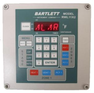
**Problem 4:** Display is stuck in either DIF, DAY, or NITE mode. **Solution:** There is damage to the board and it will need to be sent in for repair or be replaced.
