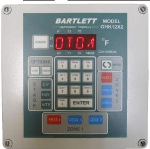
Ever turn your greenhouse temperature up temporarily and forgot to set it back? Don't wake up in the middle of the night realizing your greenhouse heat is still turned up, use the On-To-Auto feature instead.
