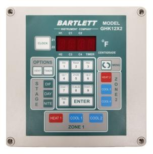
Other features include a cycle timer for irrigation, misting, or lights; a vent stage for dehumidification; an alarm output for high or low temperatures, power loss or hardware trouble; and statistics for high, low and average temperatures for the past 7 days. Our C.I.S Software is available for the option of connecting up to 99 greenhouse controllers to a personal computer for easy programming and monitoring.
