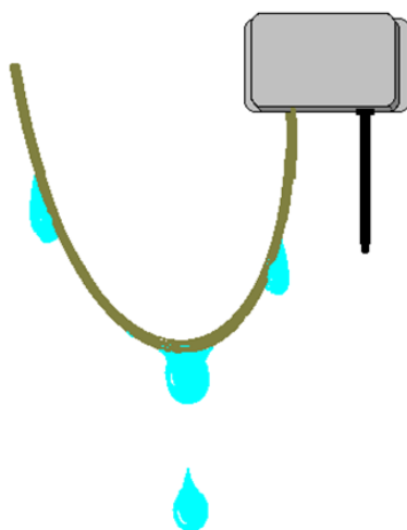
Figure 6: Example of a drip loop.
