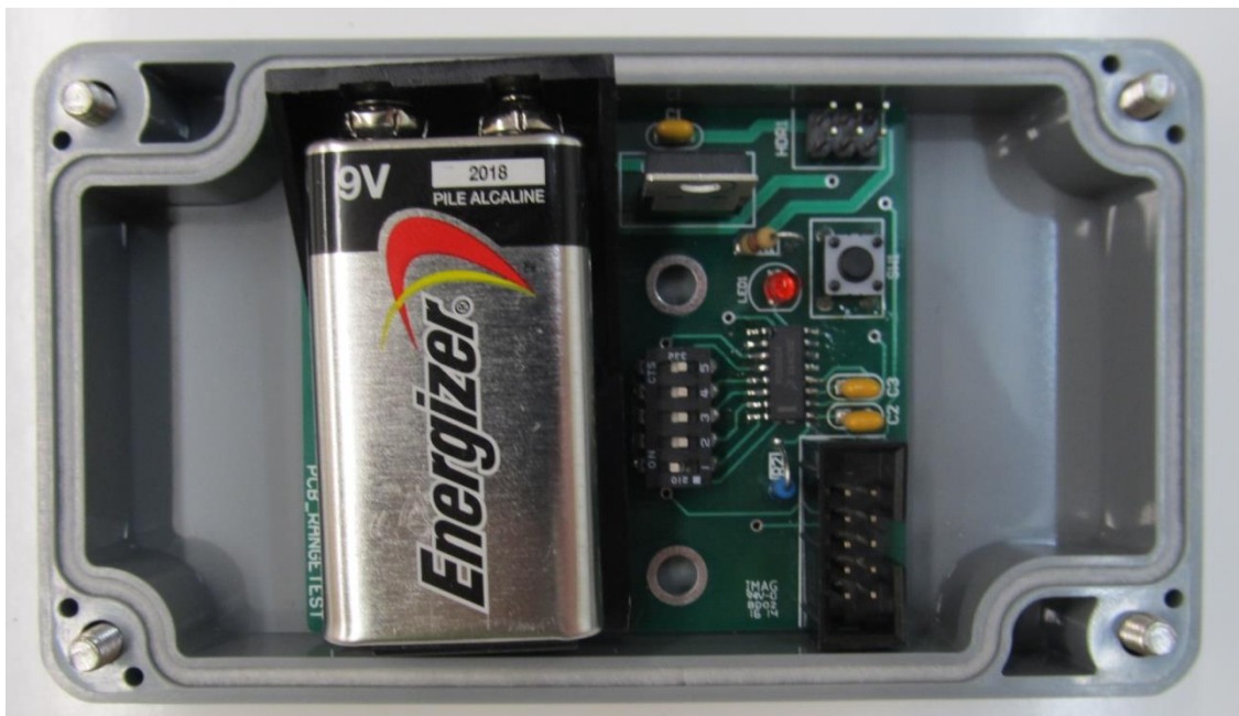
Figure 11: Range Test Board
